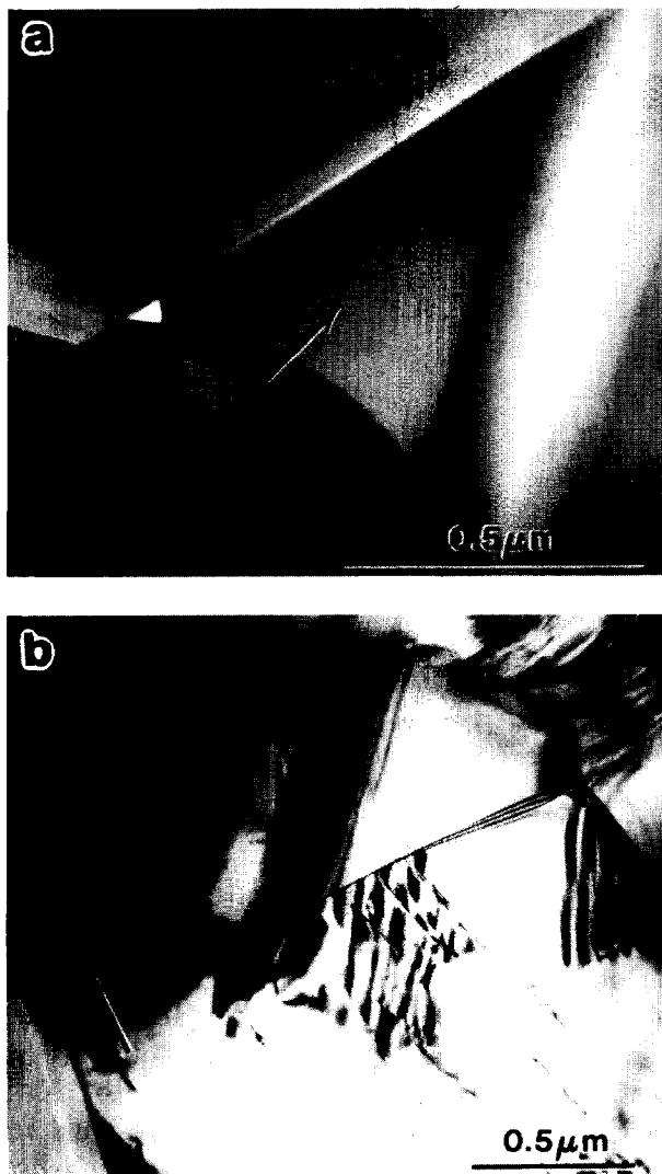
Fig. 8. TEM micrographs of interphases in \text{Al}_2\text{O}_3 -sintered \beta -SiC and its composite, (a) amorphous silica phase and (b) crystalline aluminum silicate phase.
